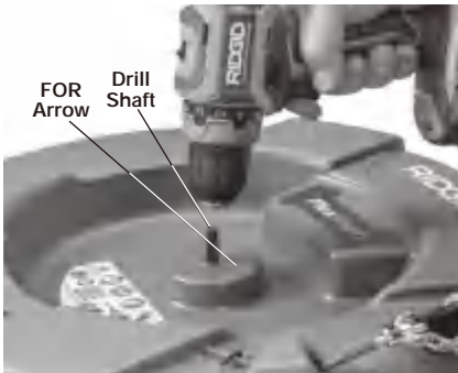
Figure 4 – Attaching Drill To Drill Shaft
